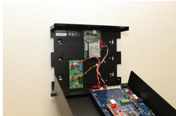
Figure 2 - Installing Main Console on Wall
